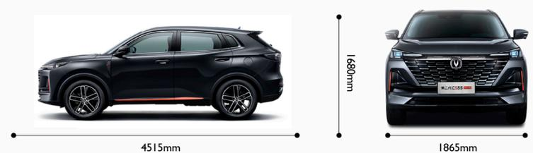
1.5 Turbo Engine NE15TGDI 2780 Wheelbase mm 188 HP 300 Maximum torque
